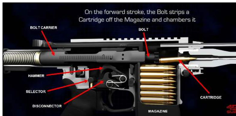
Figure 2: Post-Fire Forward Motion of Bolt Carrier 9
