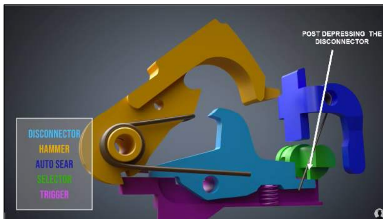
Figure 4: Firing Mechanism—M16 in Fully Automatic Mode 11
