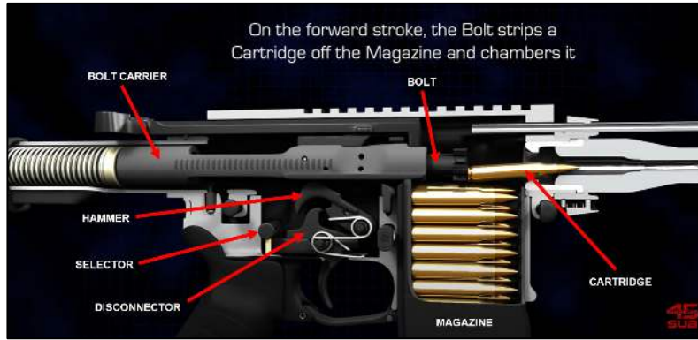
Figure 2: Post-Fire Forward Motion of Bolt Carrier 9
