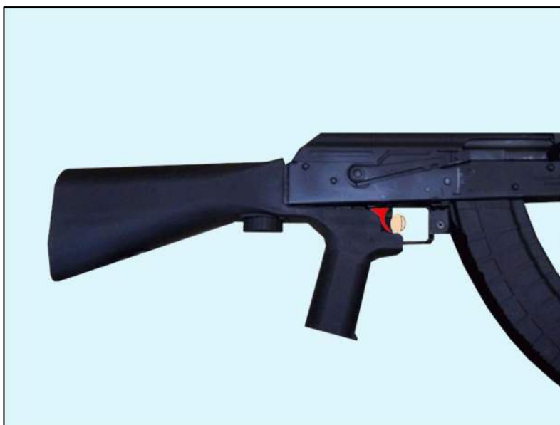
Figure 5: Pre-Firing Position of Bump Stock With Trigger Finger on Trigger Ledge 12
